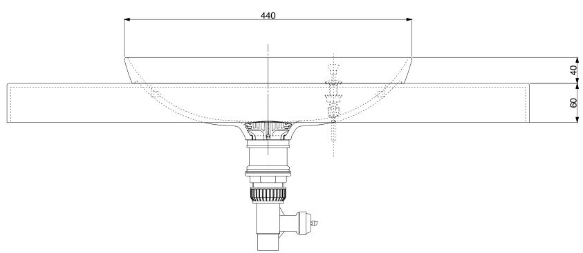
Drain Plug HV3244W2PMU2 Combined Pipe
